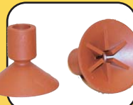
1648 MIEHLE TF and other feeders. For heavy cardboard or sheet metal. 2-1/8" high, 2-1/2" across. Fits 3/4" OD tube or 1/2" pipe. Gum rubber or Neo.
